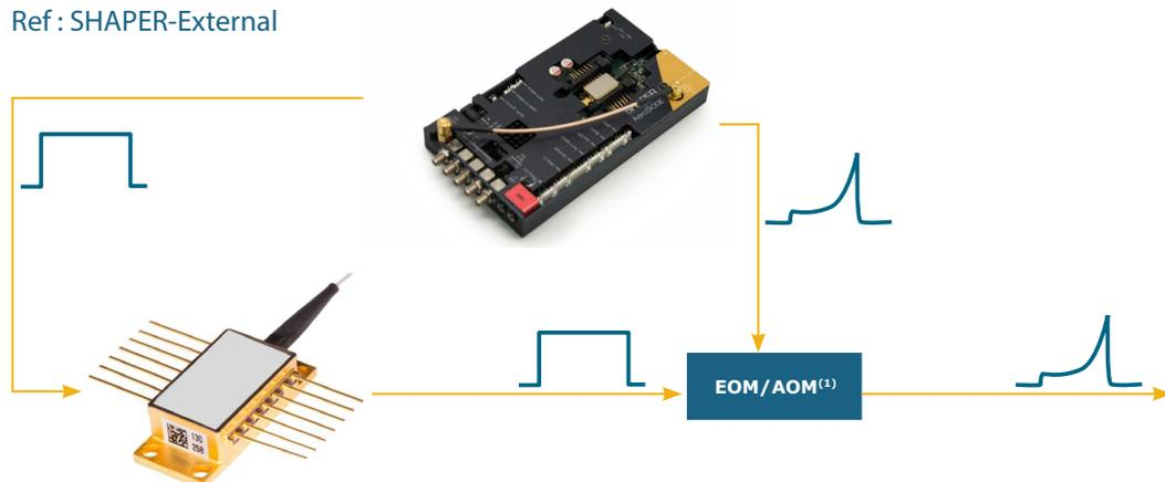
(1) Electro Optic Modulator / Acousto Optic Modulator
