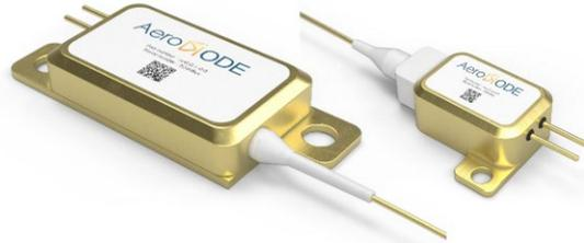
**Figure 6: Example of multimode fiber coupled laser diode pumps used in fiber lasers ( left: 150 W @ 976 nm ; right: 10 W @ 915 nm).**
