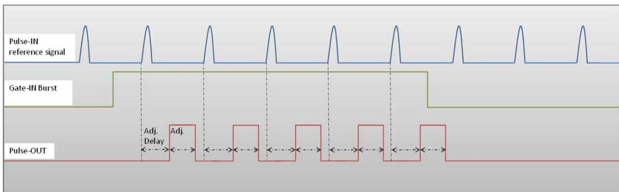
Figure 1 : Gated output from Gate-IN external signal
