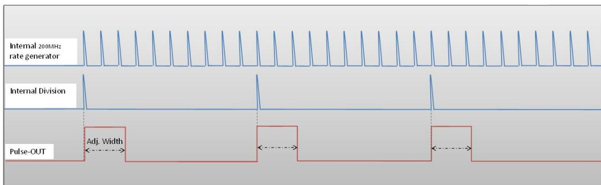
Figure 1 : internal 200MHz clock divided by 10 to get a duty cycle software adjustable 20MHz output signal
