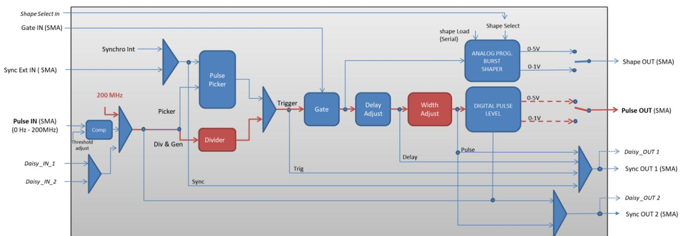
Figure 2 : Main firmware features used in Standalone Generator
