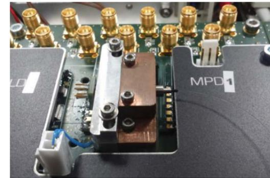
Example of butterfly (top) and TOSA (bottom) laser diode
