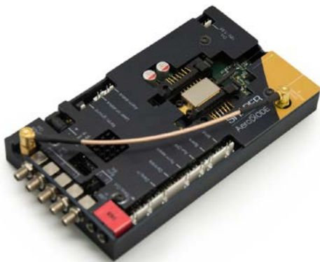
Figure 13 : AeroDIODE shaper module set in direct driver configuration (left) and special optical pulse shape obtained from a DFB laser diode after its programmed within the module (right)
