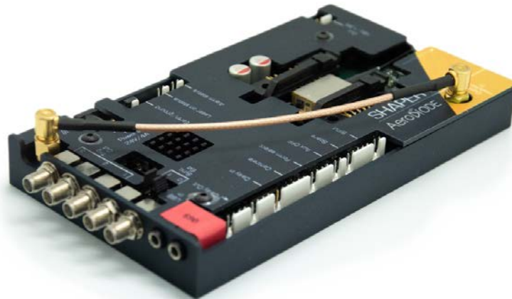
Figure 7 : Shaper board for EOM driving, combining a laser diode driver, a multiple output synchronization electronics and a 5V programmable shape output to drive an EOM with 2GHz bandwidth and 48dB dynamic range
