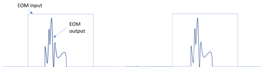
Figure 4 : Example of a pulsed configuration to overcome the average input power limitation of EOMs
