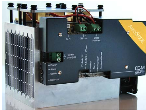
Figure 22: Aerodiode high power laser diode driver . Ideal for multi element laser diodes like II-VI , Lumentum , IPG etc.
