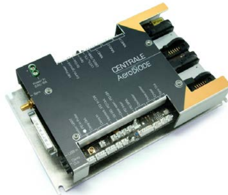
Figure 21: This fiber laser diode driver acts as a control center for fiber lasers. It includes one singlemode CW pulse driver and one nanosecond and CW laser diode driver.
