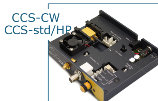
➤ Open driver for CW, std and HP electronics Boards
