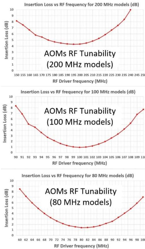
Figure 11 AOM RF tunability for each of the AOM RF frequencies (1550 nm models). Note that 200 MHz models in the 780-1100 nm range have lower minimum loss than what is shown above. The delta difference in loss when tuning the RF frequency is similar as the delta difference shown in this graph).
