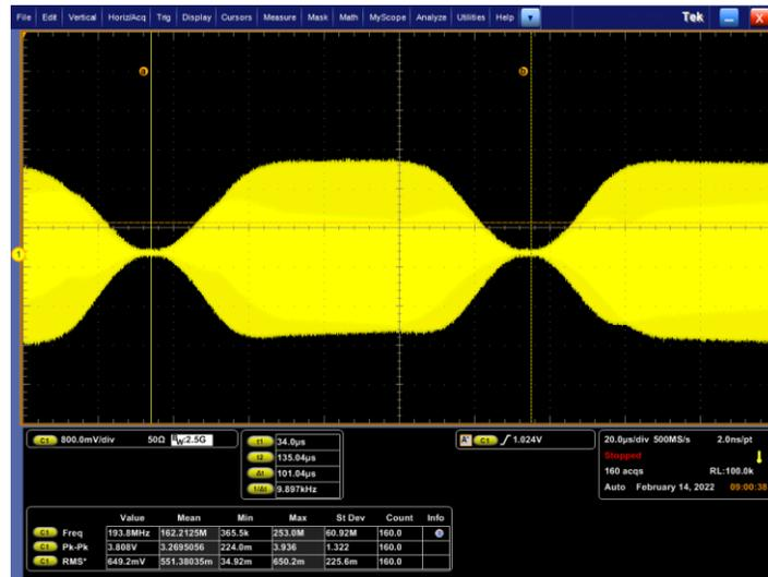
Figure 5 : Monitoring of the modulation triggering analog signal
