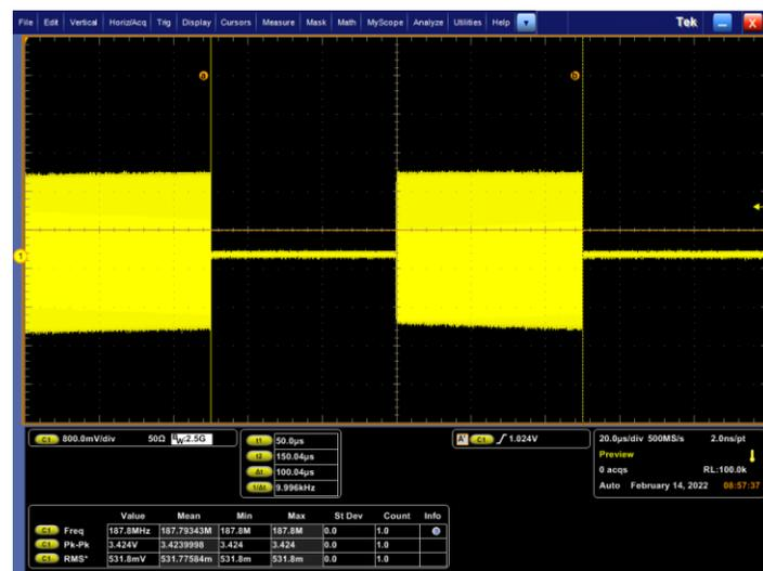
Figure 6 : Monitoring of the modulation triggering TTL signal
