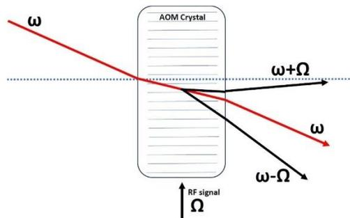
Figure 9 Diffraction principle by the AOM (acousto-optic effect)
