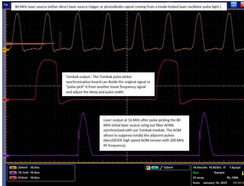
Figure 8 Pulse-picking measurement result.
