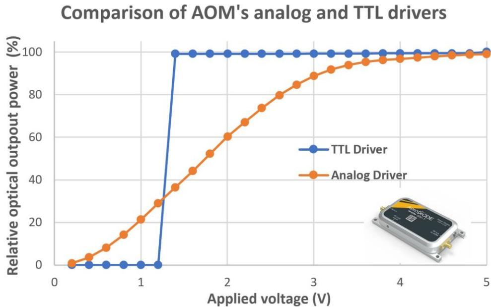
Figure 7 RF output power variation with applied modulation voltage into analog or numeric RF driver
