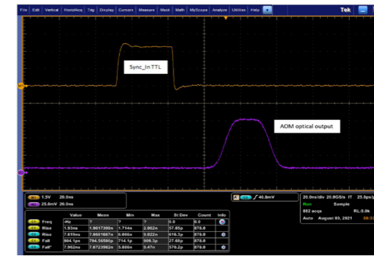
20 ns output optical pulse shape (high speed AOM version).
