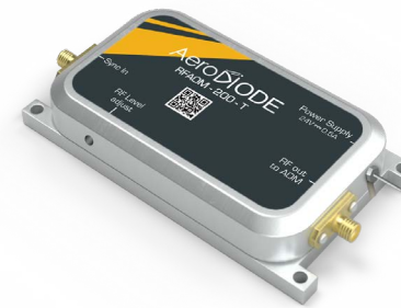
RF Driver - std version (TTL or analog).
