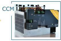
«CCM» Open-frame driver for Multimode diodes (10-200W)
