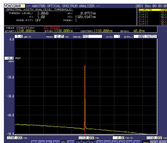
Typical spectrum of a 1310 nm DFB laser diode amplified in pulsed mode (OSA resolution 0.05 nm).
