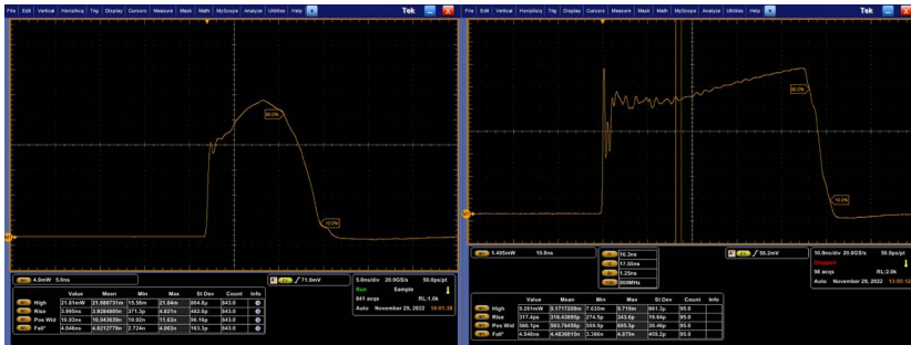
> Example of 10 ns and 100 ns pulse shapes obtained with CCS-HPP driver
