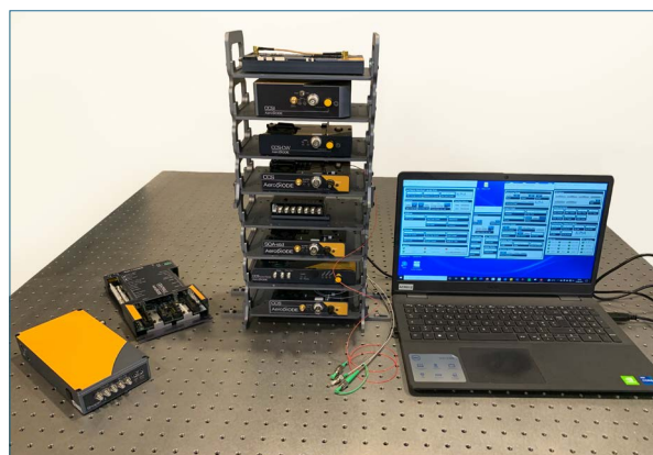
All AeroDIODE products can be connected together (daisy chain) to a unique GUI interface which consolidates all modules functions
