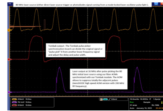
Example of a 80 MHz repetition rate input light pulse-picking down to 20 MHz.
