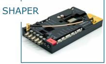
Open driver for Shaper electronics Board
