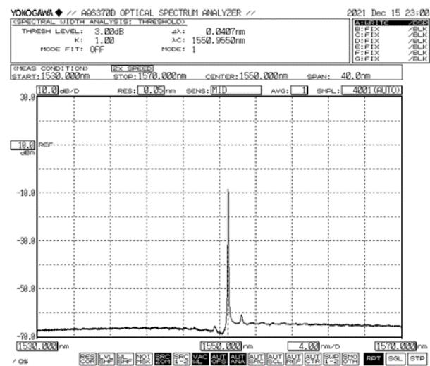
Typical spectrum of a 1550 nm DFB laser diode amplified in pulse mode (OSA resolution 0.05 nm).
